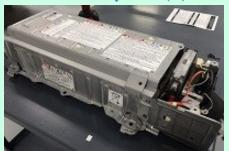
The function of the battery in an electric car is as an electrical energy storage system in the form of direct-current electricity (DC). If it gets a signal from the controller, the battery will flow DC electrical energy to the inverter to then be used to drive the motor. The type of battery used is a rechargeable battery that
