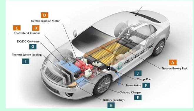
The basic main elements of electric cars installed in almost all types of electric cars are as follows:
