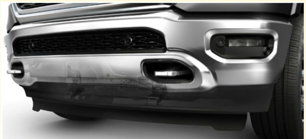
2019 Ram 1500 shows active airdam deployed. The collaboration with Magna included development of validation requirements including bench testing.
