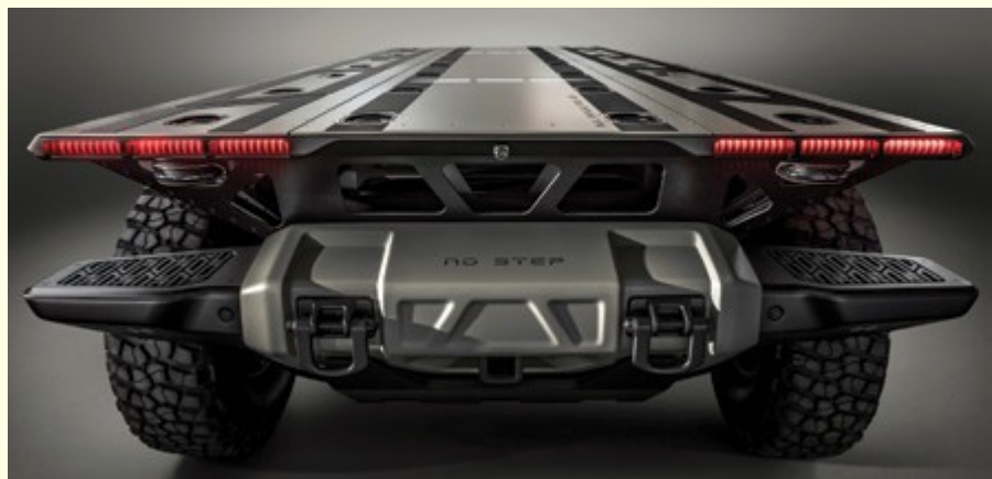
The SURUS platform includes two advanced electric drive units, four-wheel steering, advanced propulsion power electronics, a
