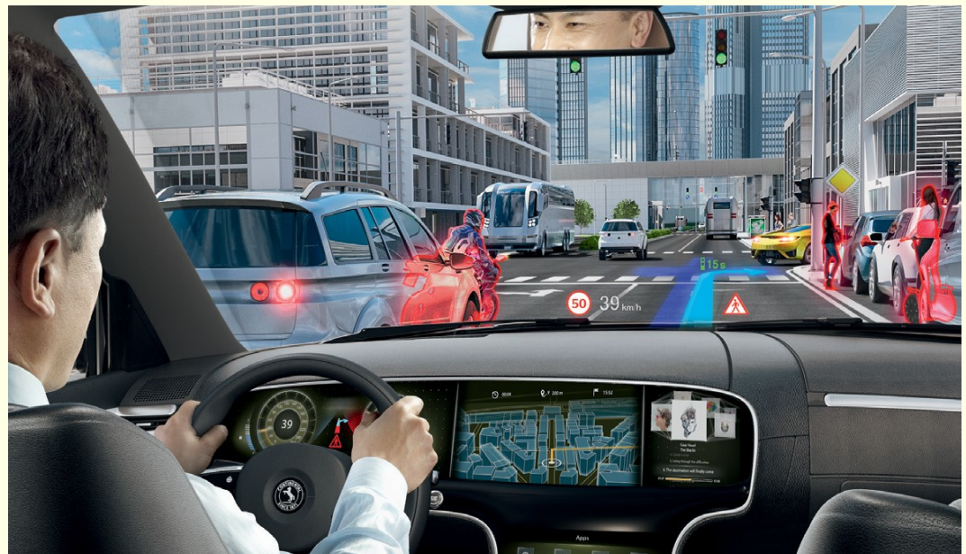
Simulation of Continental Holographic HUD technology under development, showing highlighting of a motorcyclist that's partially shielded by the SUV at left, and two pedestrians near the road at right
